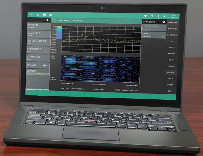
Laptop PC Running Remote GUI Application with Wi-Fi Connection to MS2080A
